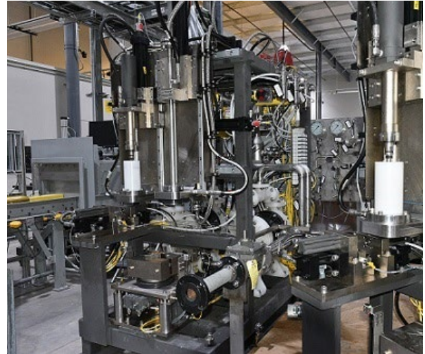
Mortar rounds first visit a station called the Munitions Washout System consisting of two Improved Cavity Access Machine arrays with four lines each.
